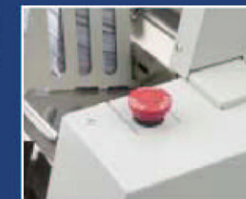
Emergency stop button for operator safety.
